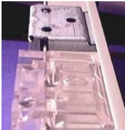
As you tighten the Screw make sure the metal tab is in the correct position. You may have to help it catch the lip of rail. *Do not over tighten the screw it will bend the tab.*
